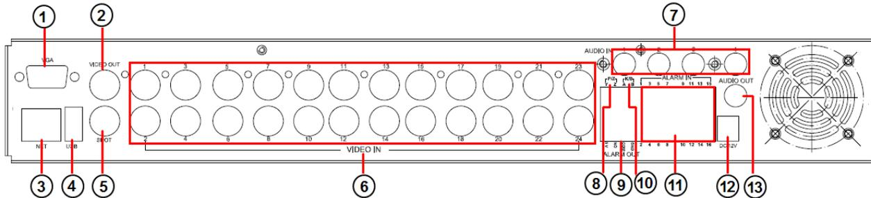
Fig 2.6 Rear Panel for 24-ch
