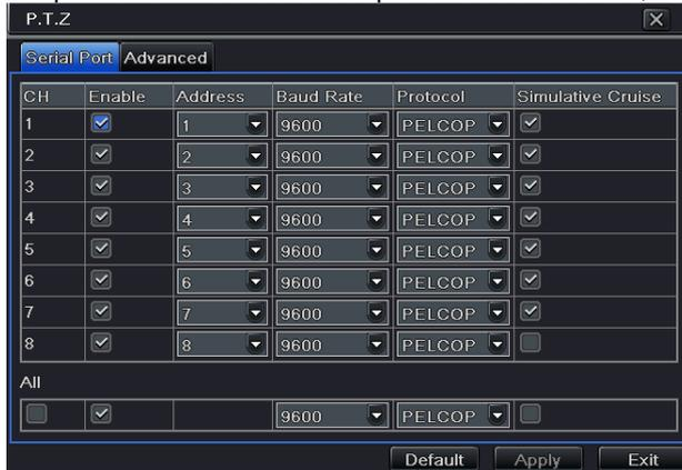
Fig 4-37 P.T.Z configuration-serial port
