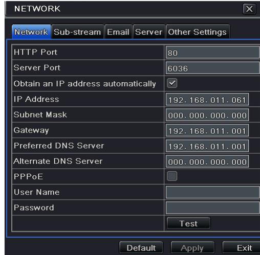
Fig 4-29 network configuration-network
