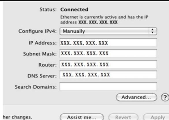
Step 3: After acquiring the IP address, Subnet Mask and so on, please enter into the DVR's Main Menu→Setup→Network interface to manually input IP address, Subnet Mask and Gateway according to the configuration of PC. The network segment should be the same as the PC. If using DHCP, please enable DHCP in the DVR and router.
