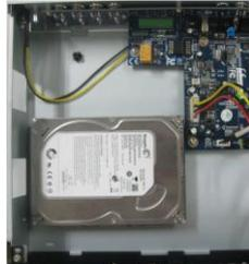
Fig 2.1 Connect HDD
