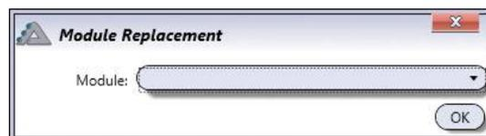
The configuration from the old module will be transferred to the new module, including the non-distributed entities (inputs, outputs, areas, tamper switches, etc.).
